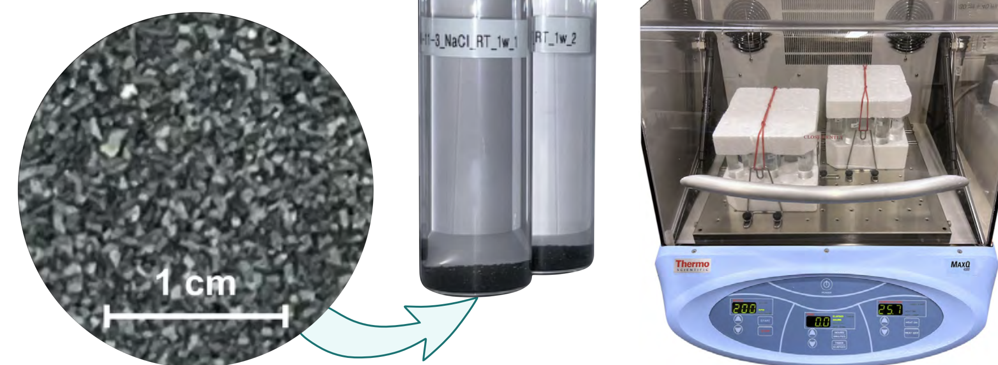
Figure 2 - Scale granulate with leachant and in orbital shaker.
