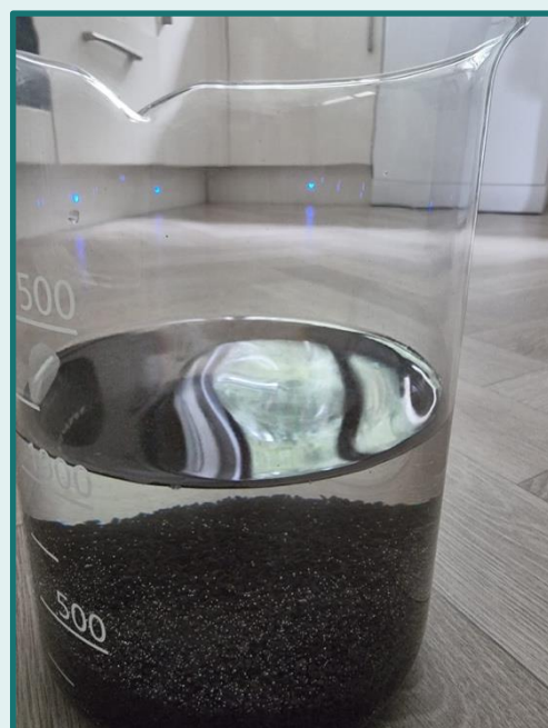
Figure 3: Equilibrating of manganese oxide on chitosan in water before application in the FluMex Miniplant.
