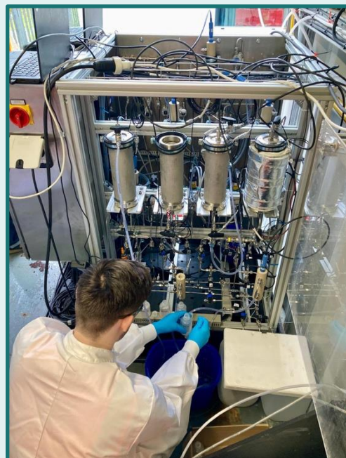
Figure 1: FluMEx Miniplant with four different columns for adsorber materials.
